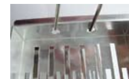
With the two holders the insert can easily be removed
